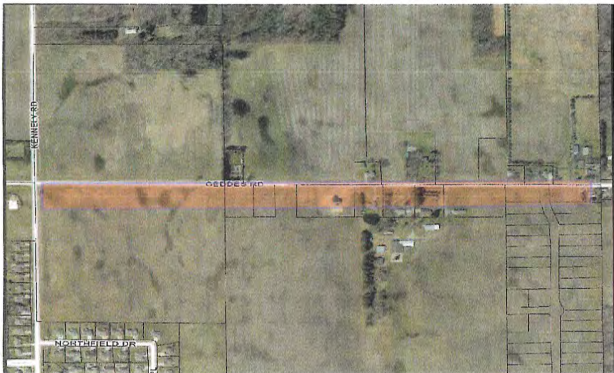
Geddes Road Gravity Sewer Route
